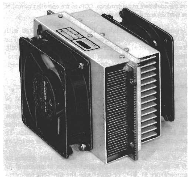
4. Cool instruments. Air-to-air thermoelectric heat exchanger cools interior of sealed electronic instrument cabinet. Exchanger is mounted through cabinet wall with its cold side facing the interior. TE modules are sandwiched between two heat sinks.
