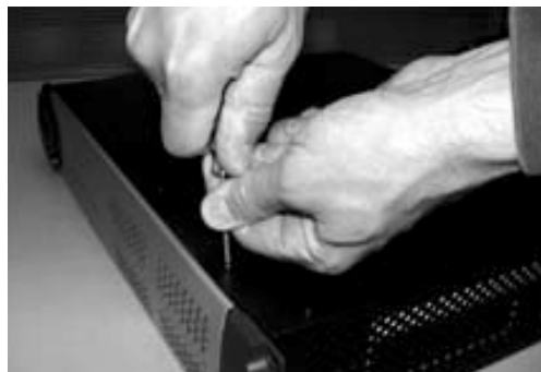
Removing the top cover screws
